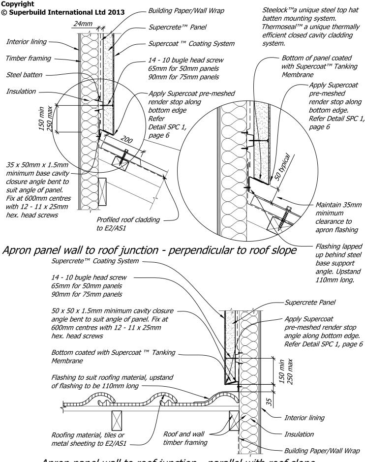
Apron panel wall to roof junction - parallel with roof slope
